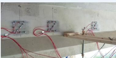
Researchers used strain gauges to determine shear distribution in prestressed concrete girders.
