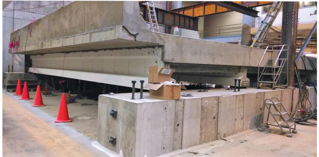
A full-scale single-span bridge with four prestressed concrete girders was constructed in the laboratory and tested to investigate shear distribution.
