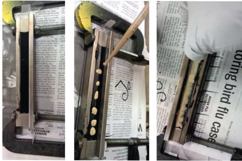
Researchers used pipettes to apply a precise amount of sealants to laboratory-created binder samples. These samples showed mild softening effects, but these impacts were not observed in samples collected from the field, so the sealants’ effectiveness is unclear.
