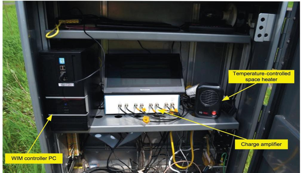
The charge amplifier compensates for temperature changes by removing slowly generated electrical charge signals from the BL sensors. But the large temperature swings experienced in Minnesota over the course of a year render BL sensors ineffective for permanent WIM sites.
