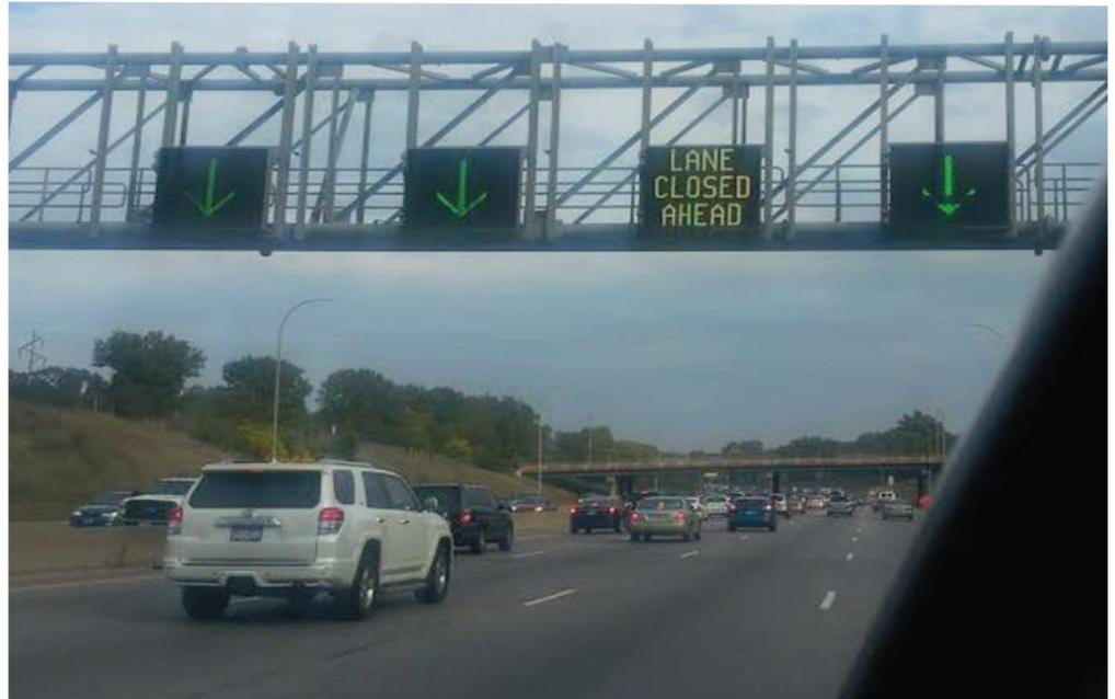
ATM signs are lane-specific and provide drivers with more detailed information about road conditions than standard changeable message signs.
