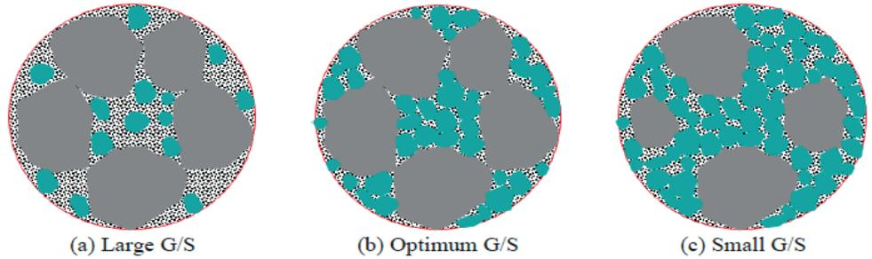
At optimum gravel-to-sand aggregate ratios, the optimized air void content maximizes stability. If the gravel content is too high (left), large air voids will cause instability and eventual deformation, while low gravel content (right) reduces durability and stability due to lack of stone-on-stone contact.
