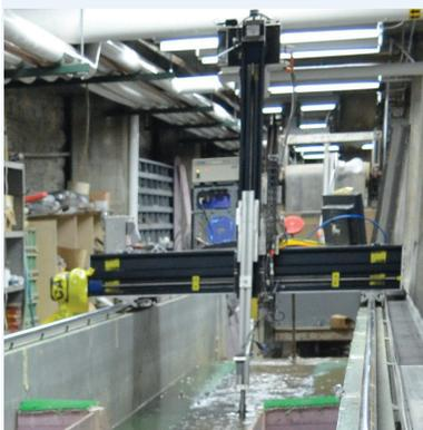
Instrumentation in the tilting flume in the laboratory collected water flow measurements.
