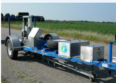
Carried via trailer, a falling weight deflectometer measures pavement response to loads.
