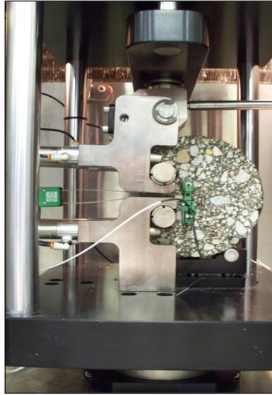
Researchers evaluated core samples from test sites for their resistance to cracking using the disk-shaped compact tension test in which a specimen is loaded to failure.
