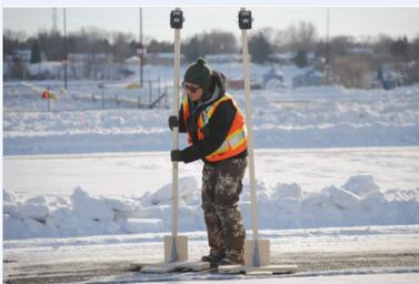
Pole-mounted time-lapse cameras with detachable bases documented deicer and plow testing on side-by-side test tracks.
