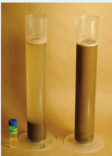
Adding flocculant (left) to a sample of water from the Minnesota River causes sediment to clump and sink.
