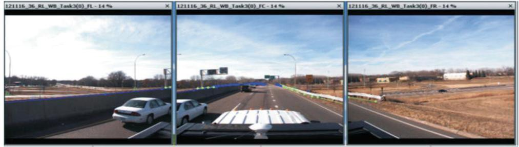
The extraction process from mobile imaging triangulates the location of barriers and other assets by comparing the items in consecutive images. These images also show attributes such as attached items, materials, barrier height and barrier condition.
