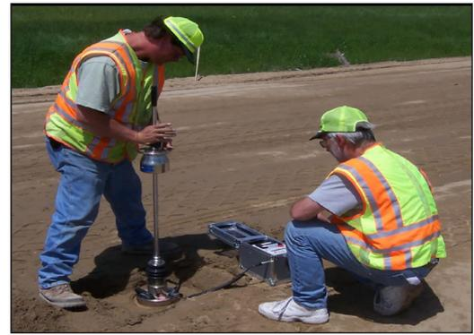
Researchers established models that will help determine the effects of moisture on the results of tests using the lightweight deflectometer (left). The LWD can be used in the field (right) to assess a foundation material’s stiffness by measuring deflections in response to a dropped weight.
