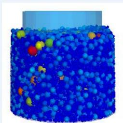
Researchers created a three-dimensional computer model simulating the interaction of an LWD loading plate with aggregate particles.
