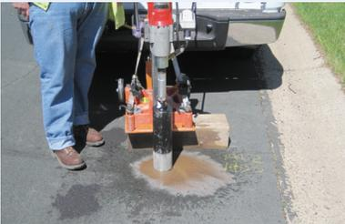
Researchers took core samples of city streets for air void and permeability testing in the laboratory.
