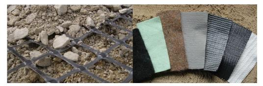
Where geogrids (left) consist of polymers such as polyester or polystyrene formed into open grids that provide support, geotextiles (right) have the quality of woven fabrics, making them good solutions for facilitating separation, filtration and drainage.
