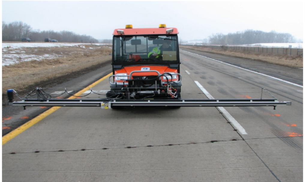
To verify results for back-calculating curl from FWD measurements, researchers compared it to an alternative method involving backcalculation from surface profiling.
