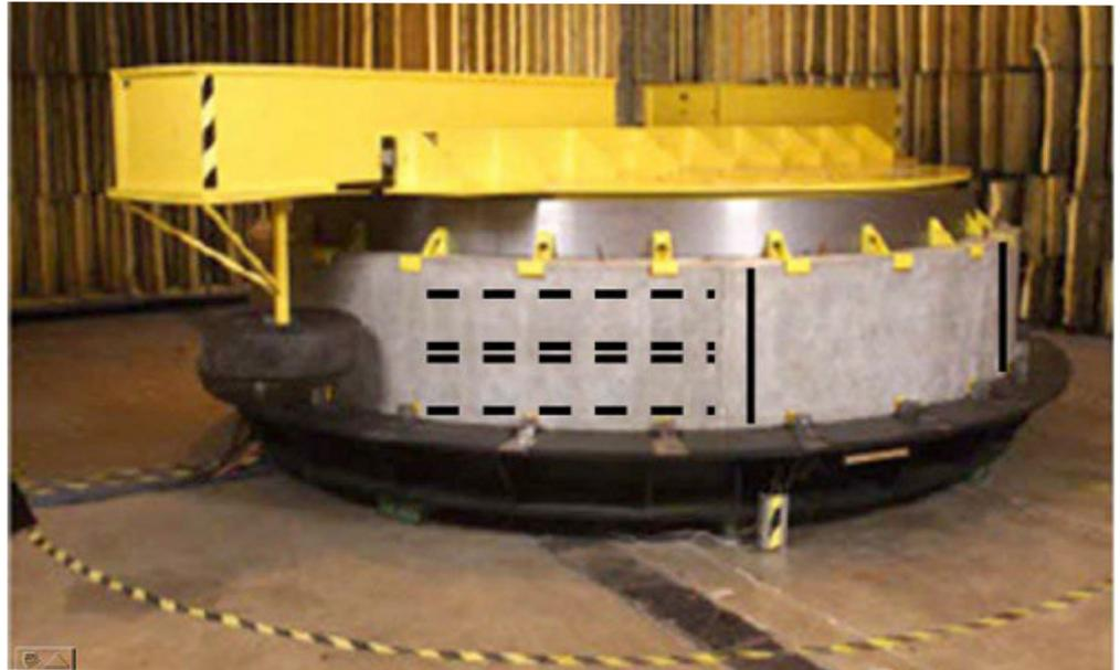
The innovative and ultimate grinds were developed and evaluated in the laboratory using Purdue's Tire Pavement Test Apparatus, a 12-foot-diameter rotating drum to which pavements can be attached and moved relative to a tire or grinding head at 30 miles per hour.
