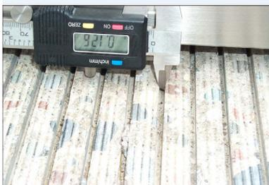
The ultimate grind was developed to improve the friction of the innovative grind by using wider, corrugated fins.
