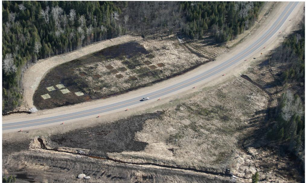
As shown in this aerial photo taken after project completion, two gravel pit basins were used, one on each side of the road. This site was chosen for its proximity to existing shrub swamp, wooded swamp and bog wetlands as well as the organic donor soil used for this project.
