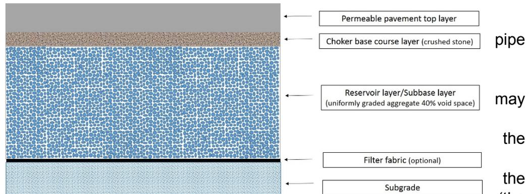
Figure 1: Permeable pavement layers
