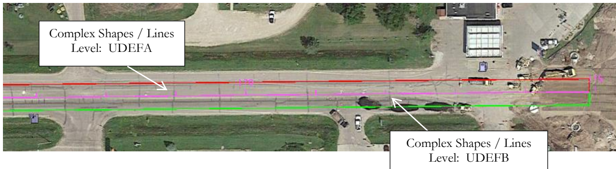
Figure 7.14. Snapshot of complex shapes / lines for 18-ft paving (1.5 lanes).
