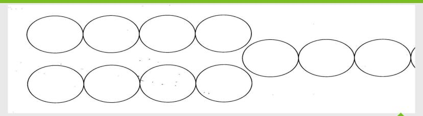
This is how we show IMPACT ATTENUATOR BARRELS on the plan. They are paid for by the EACH, we do not pay for barrels as assemblies.
