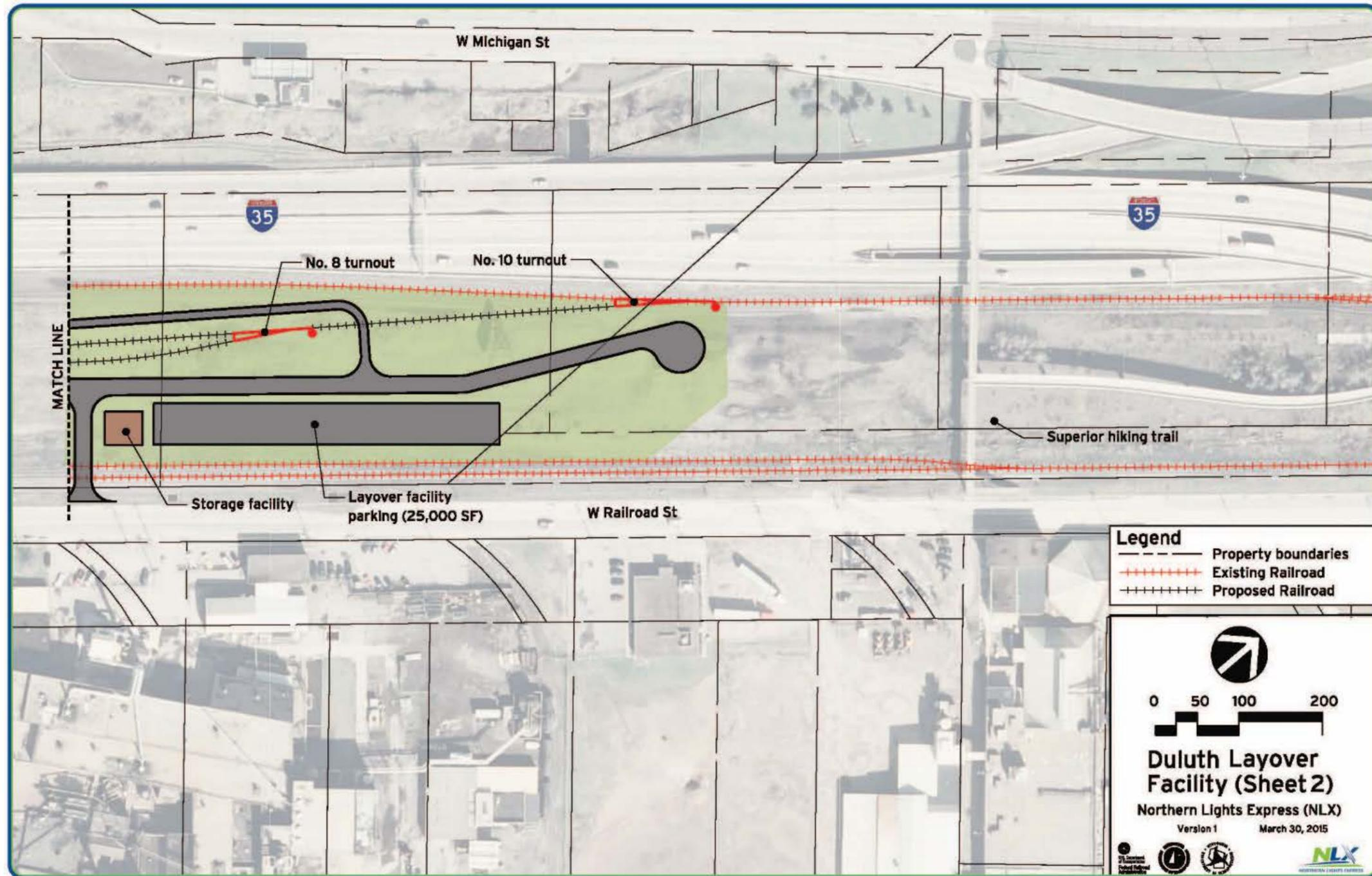
Figure 2-27: Duluth Maintenance Facility (1 of 2)
