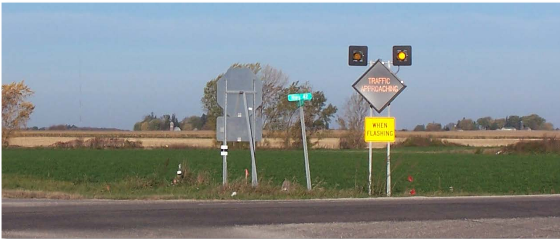
Figure 15: Rural intersection conflict warning system (RICWS) sign
