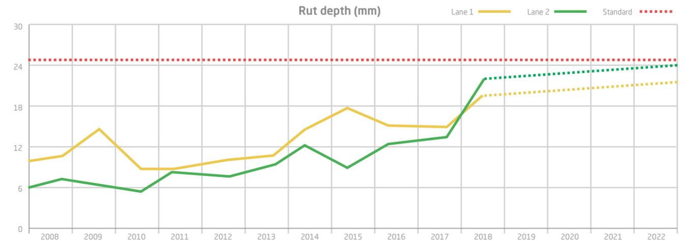
Fig. 1: Rut depth development and expected life span of Fv 181-01 Eidsbygda-Nordvika
