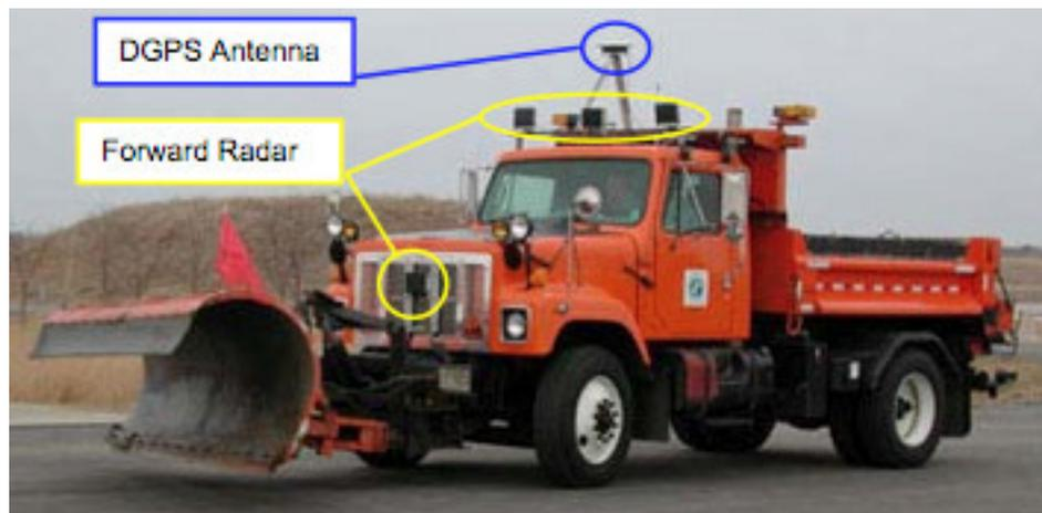
**Figure 2. MnDOT snowplow equipped with DAS technologies (from MnDOT 2004-09)**
