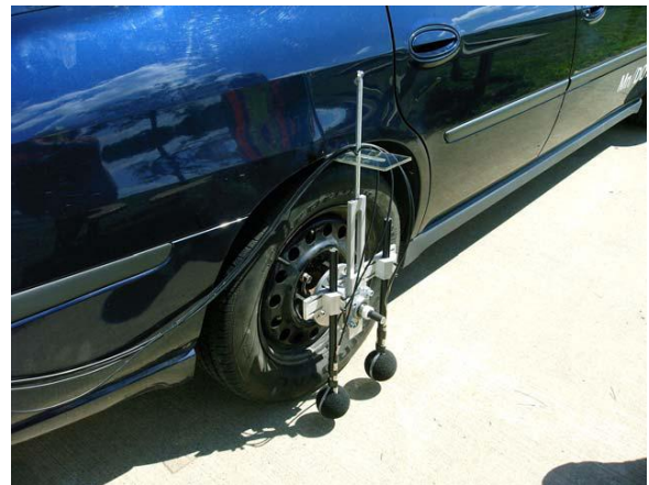
OBSI Setup. The front end is connected to these intensity probes via cables.
