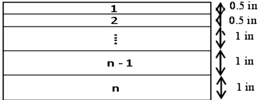
$$Z_{eff} = \sum_{i=1}^{k-1} h_i \sqrt[3]{\frac{E_{AC,i}}{E_{subgr}}} + \frac{h_k}{2} \sqrt[3]{\frac{E_{AC,k}}{E_{subgr}}}$$
