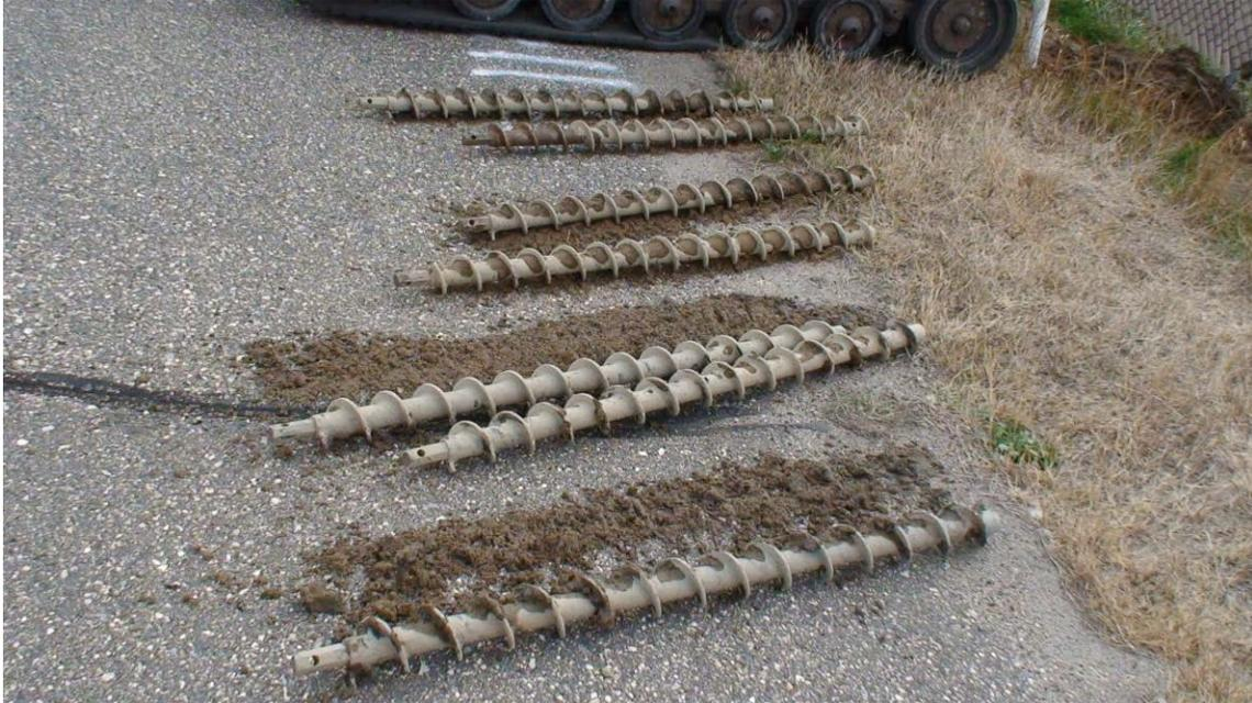
**Figure 2.12: Well 2 Encountered Saturated Sands up to 30 ft Depth Below Surface**
