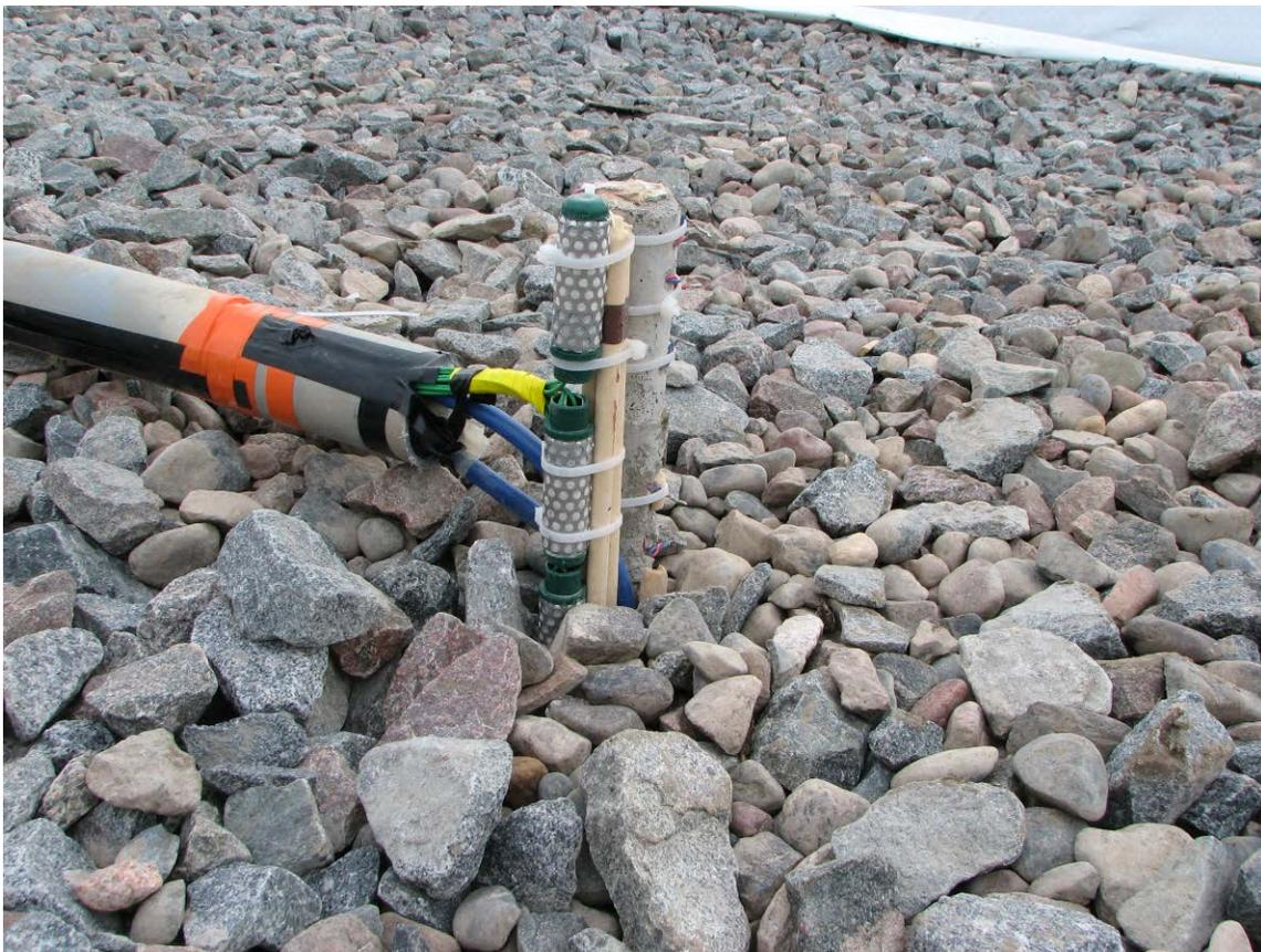
**Figure 5.6: Water Mark on Cell 85. Installed to 6-ft Below the Surface**
