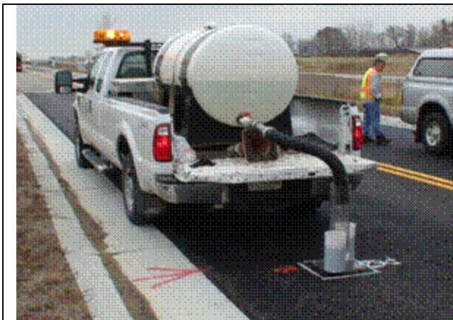
**MnDOT Infiltrometer Test**
