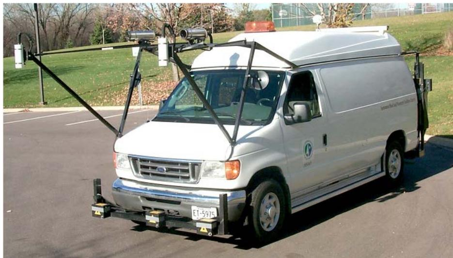
**Figure 6.2: Digital Inspection Vehicle**
