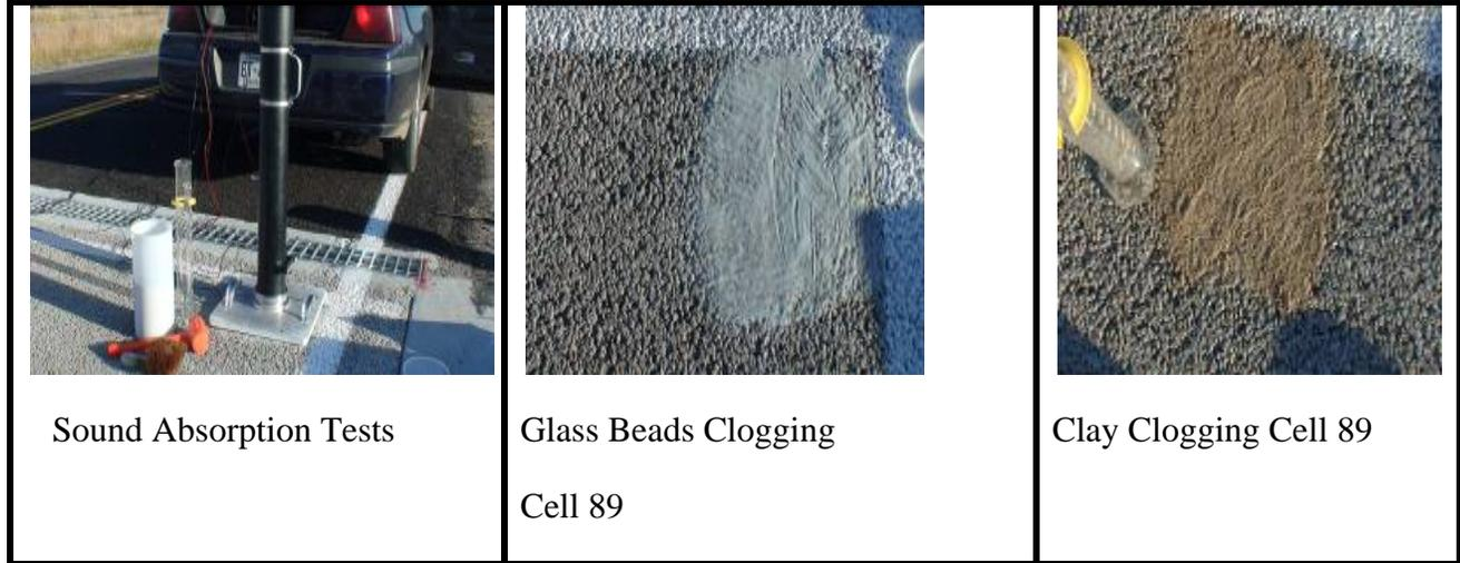
**Figure 9.7: Accelerated Clogging Test**
