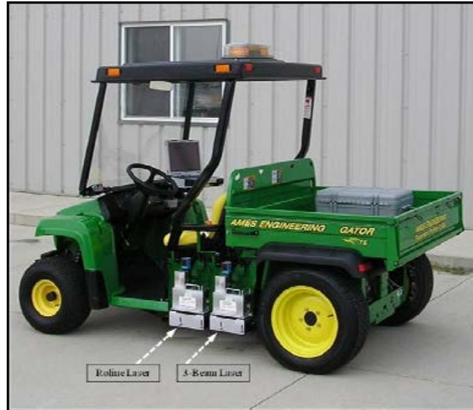
**Figure 6.1: Lightweight Inertial Surface Analyzer**
