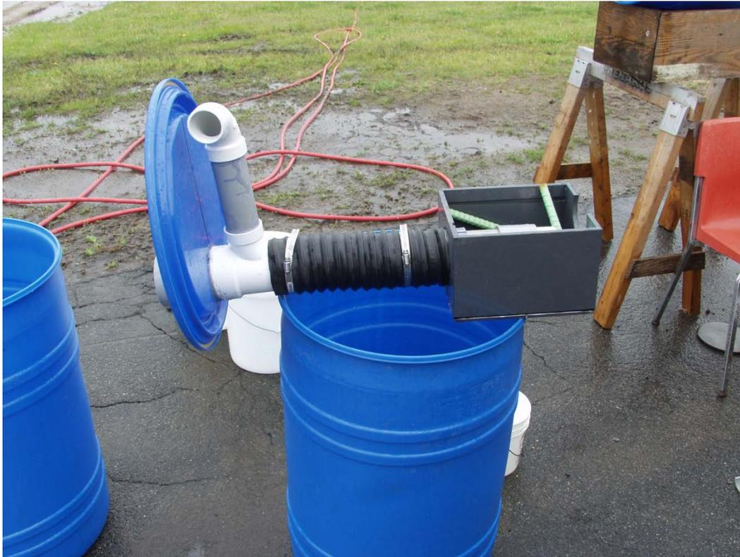
**Figure 5.3: Transverse Drain and Flow-out Meters**
