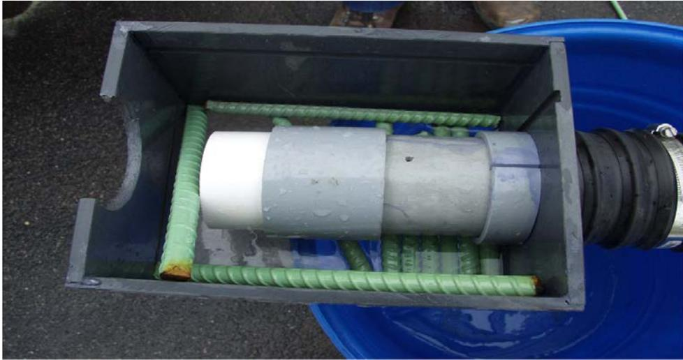
**Figure 5.4: Flow Out Meter Partial Assembly**
