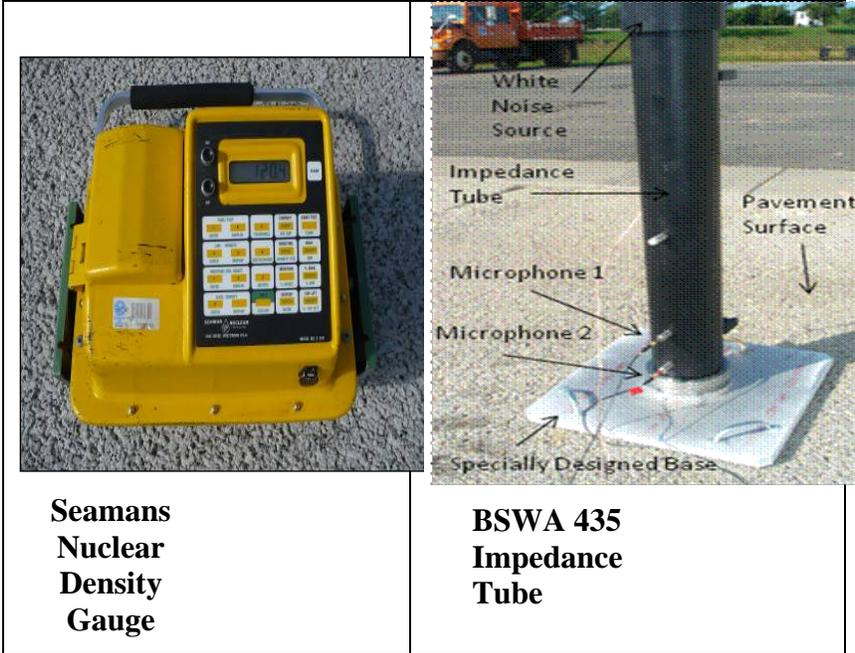
**Figure 9.5: Nuclear Gage and BSWA 435 Sound Absorption Impedance Tube**
