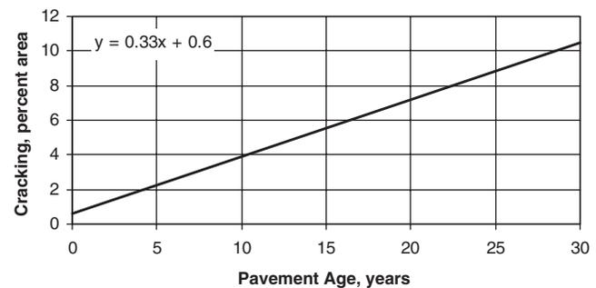
Figure 15. Assumed cracking do-nothing curve for Case Study 1—Arizona.
