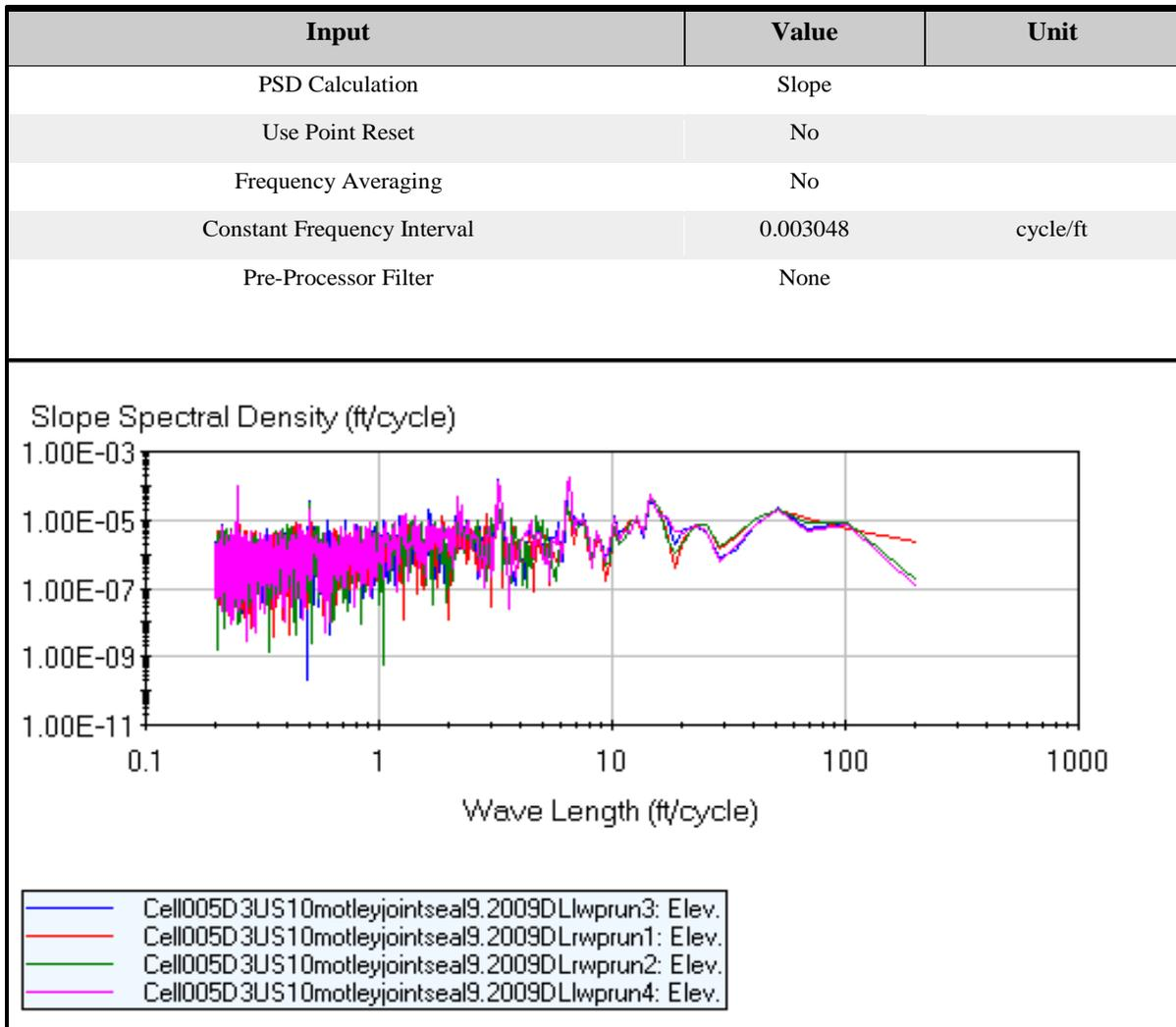
**Figure 9: Analysis - Power Spectral Density in Cell 5**
