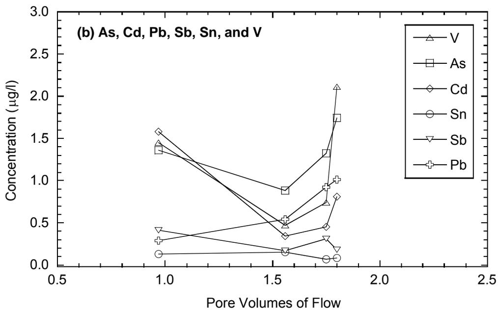
Fig. 11 Concentrations of trace elements in leachate collected in lysimeter in Waseca: (a) elements with peak concentrations between 3 and 102  $\mu\text{g/L}$  and (b) elements with peak concentrations less than 2.5  $\mu\text{g/L}$ .
