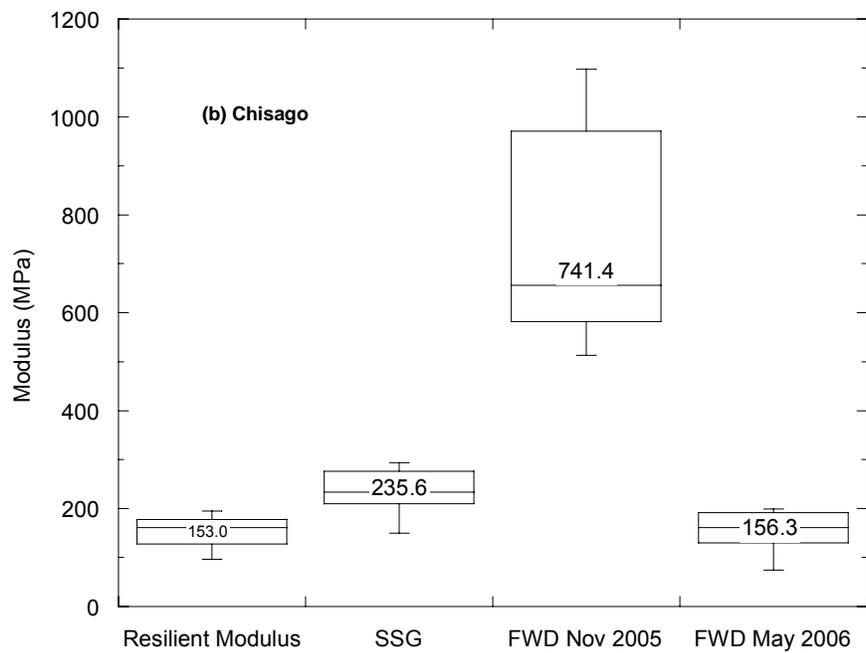
Fig. 4 Modulus as determined by different methods (numbers on the boxes indicate mean modulus)
