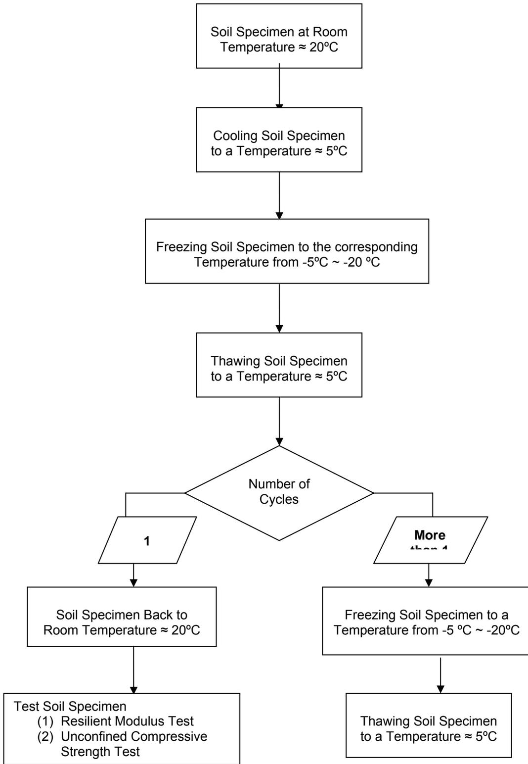
Fig. 5 Description of the process used for freeze-thaw cycling
