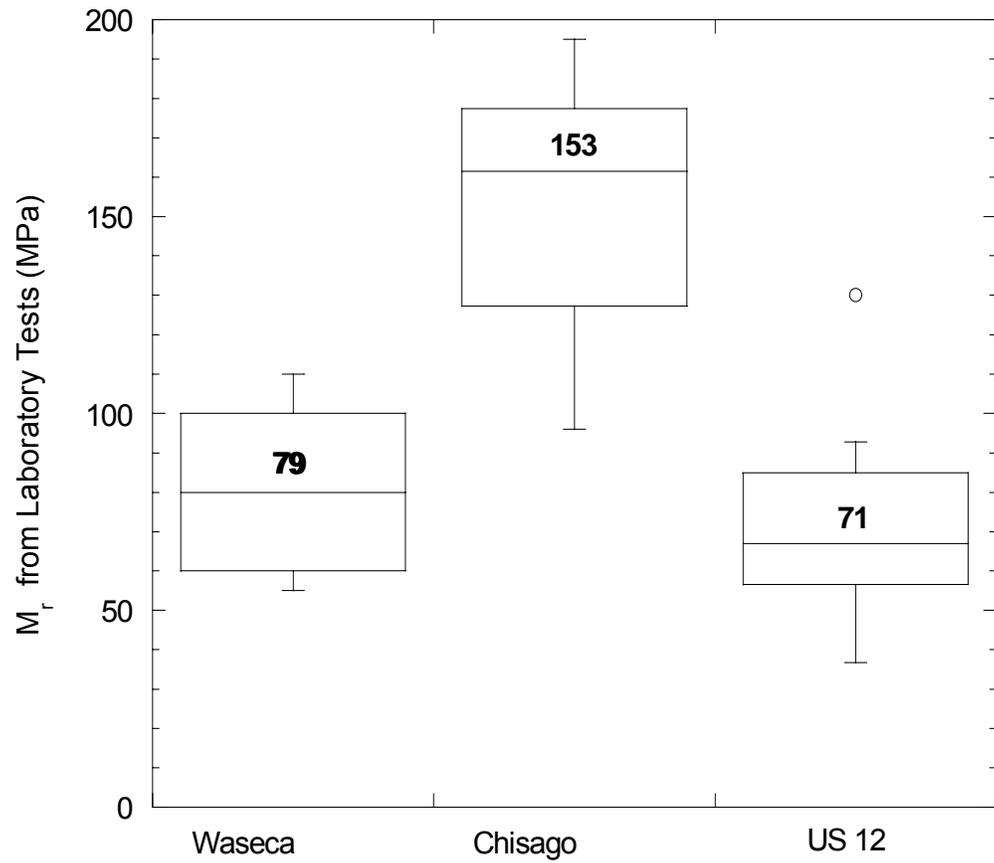
Fig. 1 Laboratory  $M_r$  of field-mix fly ash-stabilized materials (numbers on the boxes indicate mean modulus)
