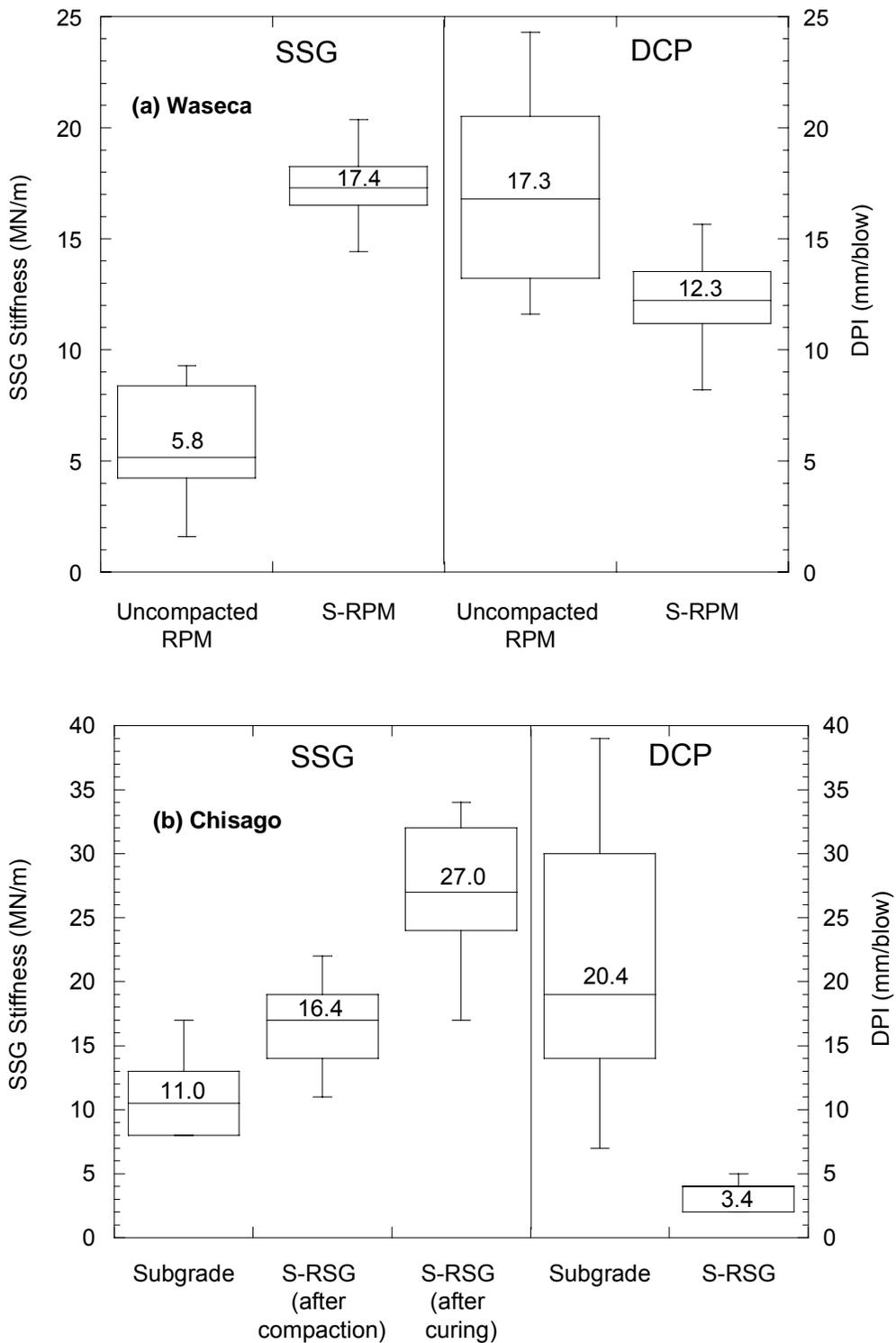
Fig. 2 Stiffness and DCP of base material and fly ash-stabilized recycled pavement material and road surface gravel (numbers on the boxes indicate mean value)
