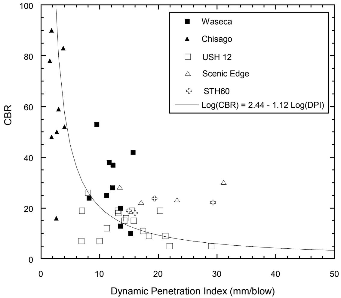
Fig. 9 CBR versus DPI for fly ash-stabilized materials
