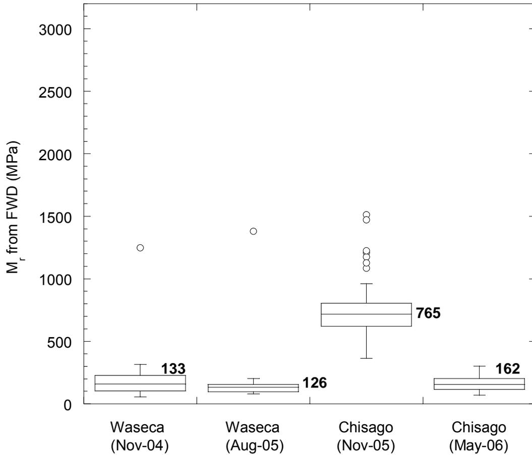
Fig. 3 Back-calculated  $M_r$  of fly ash-stabilized layer from FWD data at Waseca and Chisago projects (numbers on the boxes indicate mean modulus)
