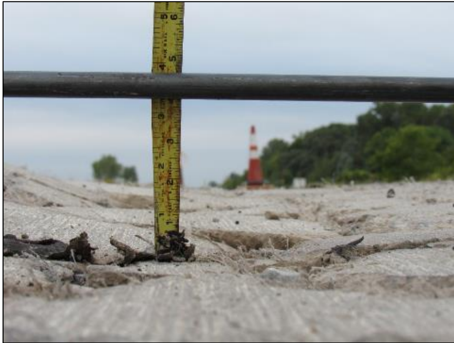
Figure 2-4. Depression along the wheel path in Cell 139 .
