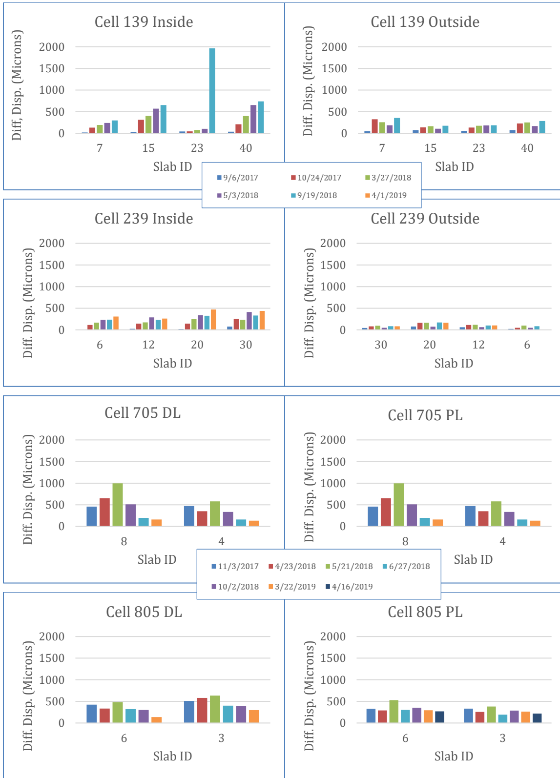
Figure 4-3. Differential displacement of Cells 139, 239, 705 and 805.
