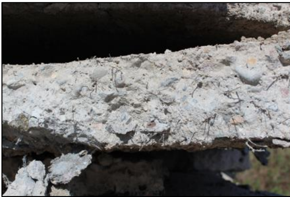
(2.5c) Fibers on the fractured face of a concrete piece.
