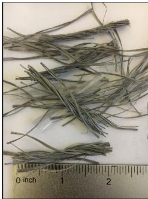
Figure 1-2: Photograph of the Forta Ferro fibers used in MnROAD 2017 FRC research cells.
