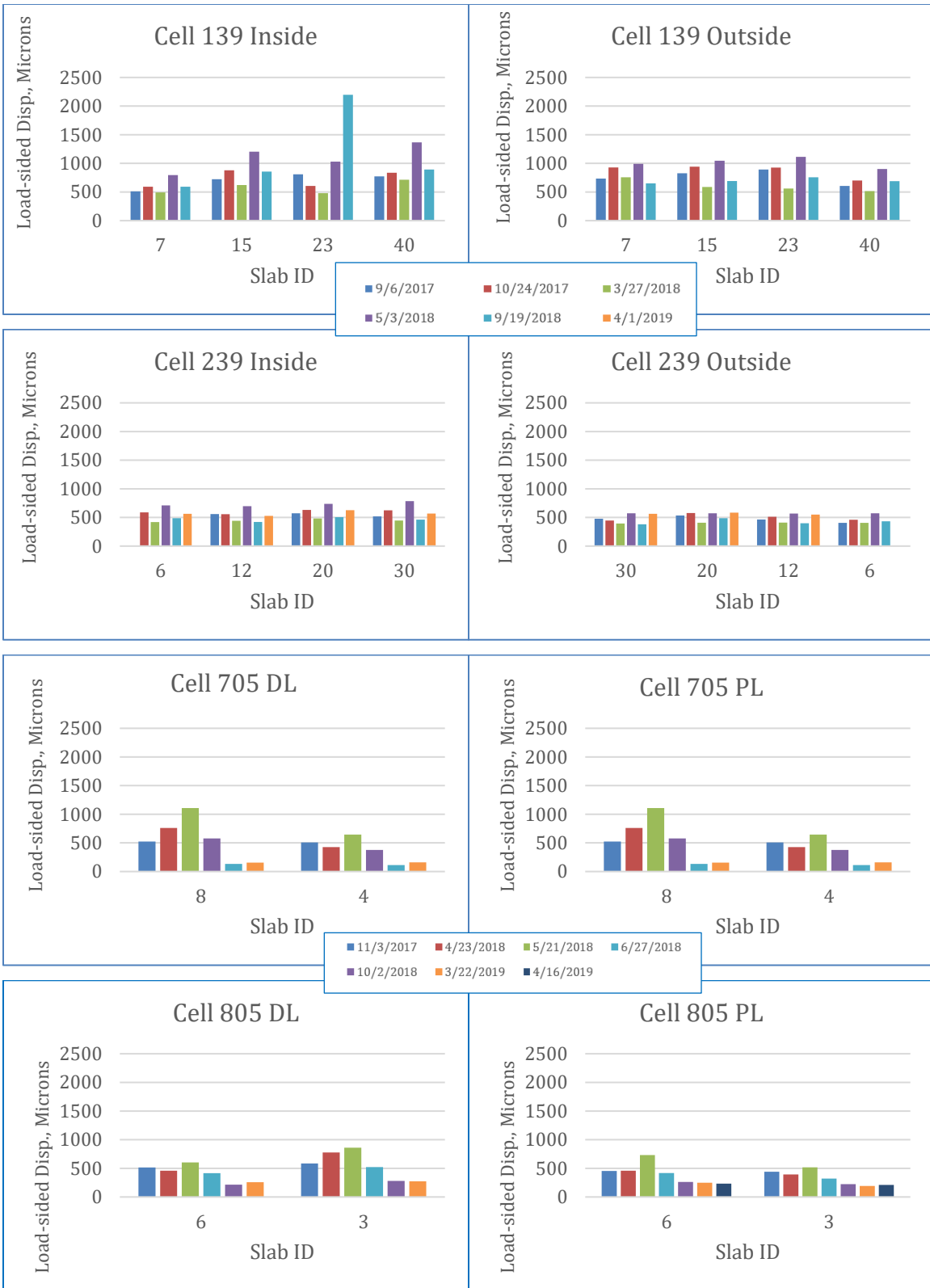
Figure 4-5. Load-sided Displacement of Cells 139, 239, 705 and 805.
