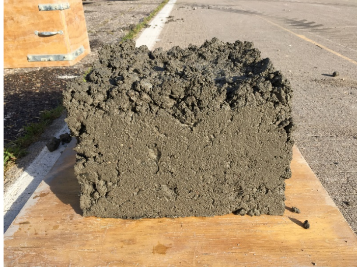
Figure 5- Box test showing voids on concrete surface
