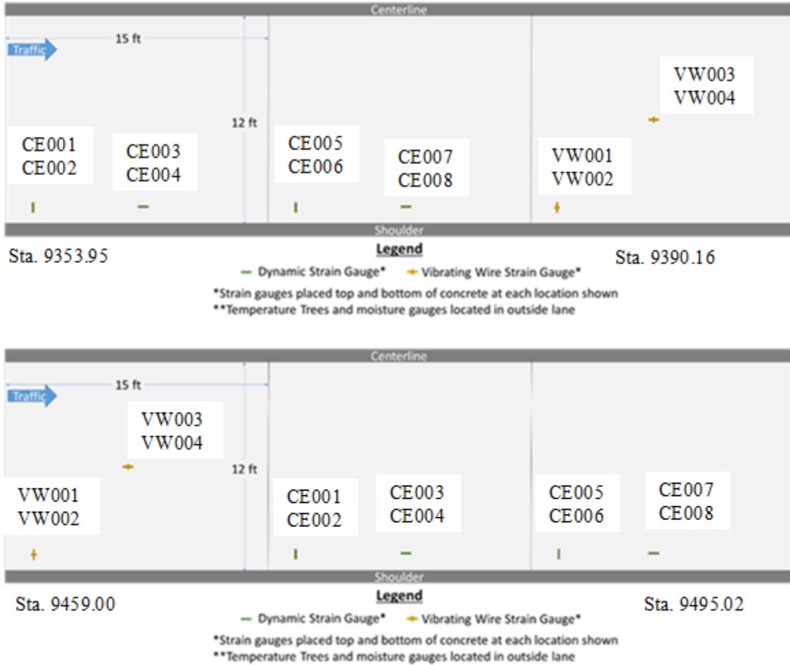
Figure 10- Sensor installation plan for cell 138 (top) and cell 238 (bottom).
