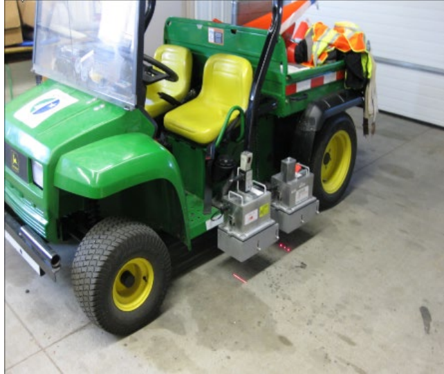
Figure 15- MnDOT's Lightweight Profiler
