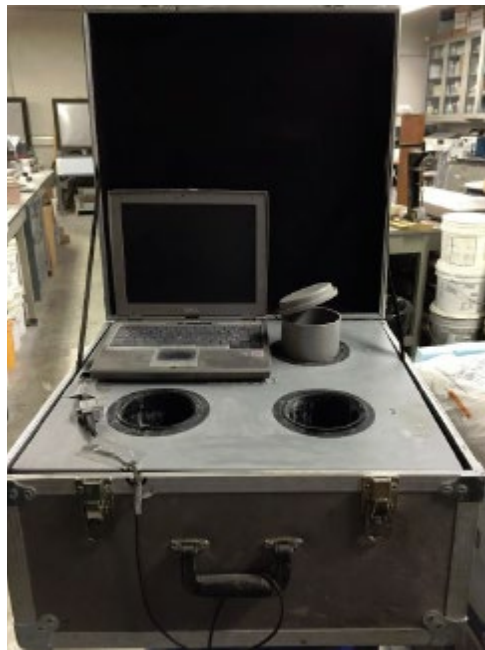
Figure 6- Calorimetry test setup for measuring the heat of hydration
