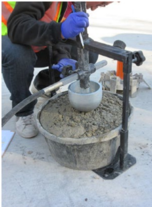
Figure 4- VKelly test setup
