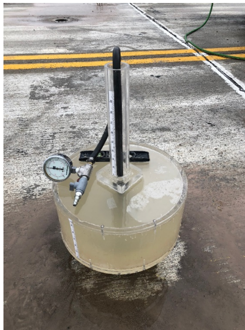
Figure 27- Borehole permeability test setup
