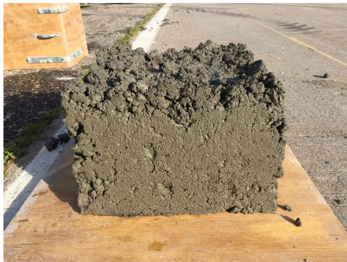
Figure 5- Box test showing voids on concrete surface
