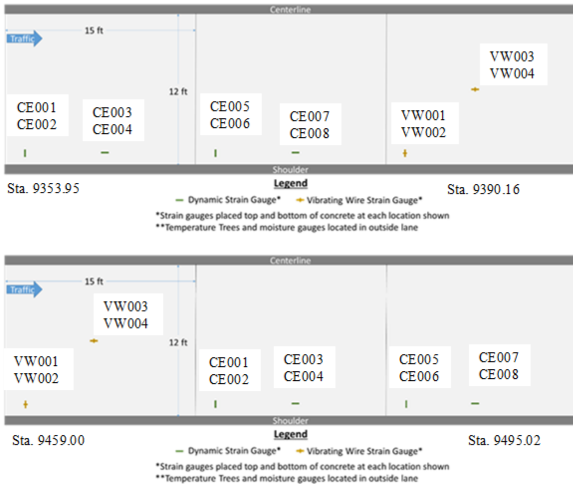
Figure 22- Sensor installation plan for Cell 138 (top) and Cell 238 (bottom).
