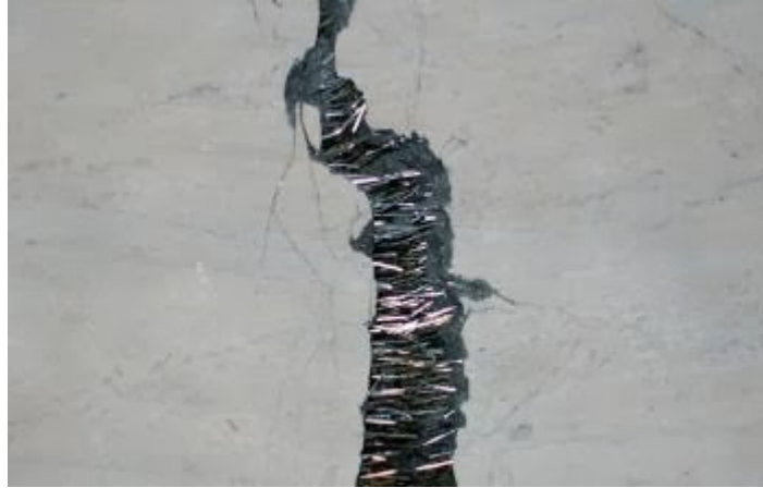
Figure 2-1. Fibers bridging a crack and providing post-crack performance (Gaddam, 2016)
