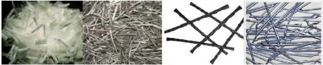
Figure 3-3: Fibers used in the (Kevern et al., 2016) study: polypropylene fibrillated fiber (left), polypropylene macro fiber (left middle), carbon fiber (right middle) and steel fiber (right)
