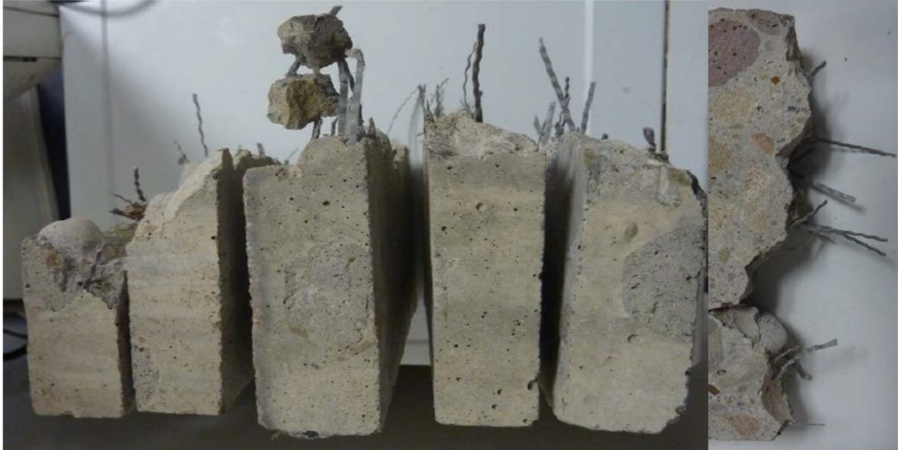
Pictures of Enduro 600 fibers after fatiguing with 10 million load cycles.
