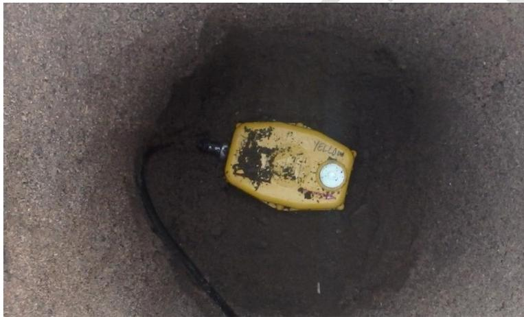
Figure 3.5. Geophone installed in a borehole (Van Deusen et al. 2018)
