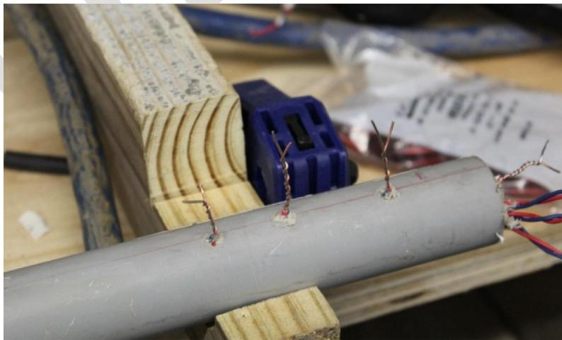
Figure 3.2. Thermocouple array in the PVC pipe (MnDOT 2014a)
