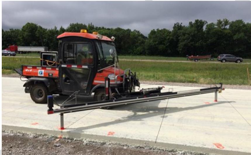
**Figure 3.7. Automated Laser Profile System (ALPS) device (Van Deusen et al. 2018)**
