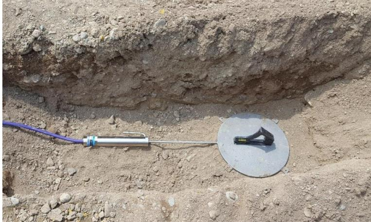
Figure 3.4. Placement of Geokon 3500 dynamic pressure cells (Van Deusen et al. 2018)
