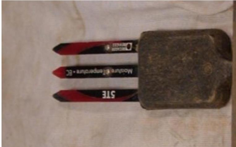
**Figure 3.3. Decagon 5TE moisture probe (MnDOT 2014b)**
