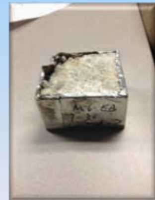
Typical concrete scaled surface profile after 80 F-T cycles
