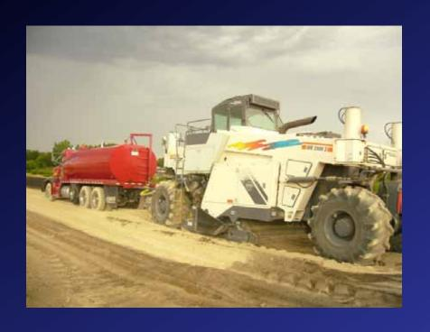
Reclaimer used for prepulverization, emulsion addition, and fly ash stabilization of Cell 4 subgrade
