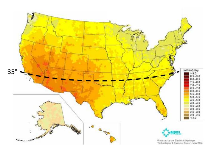
150 m<sup>2</sup>/person x 5 kWh/m<sup>2</sup>/day x 0.1 conversion efficiency = 75 kWh/person/day
