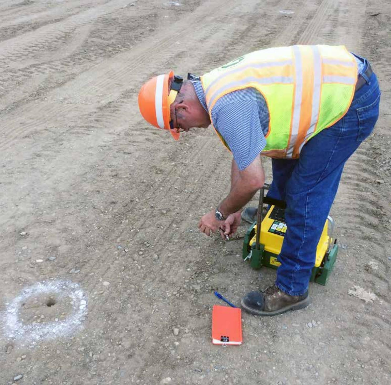
MnDOT Materials Office's Eddie Johnson uses nuclear density meter to check compaction of test cell base material before pavement overlay is placed.
