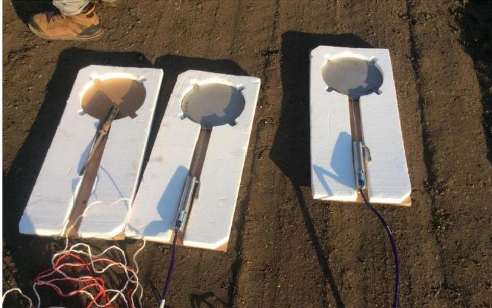
Figure 2: Organizing Pressure Gauges Before Installation
