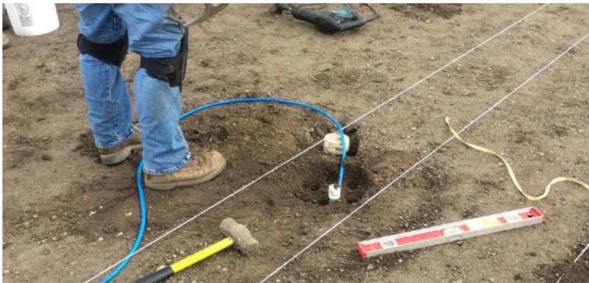
Figure 9: Thermocouple Installation
