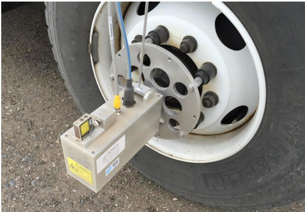
Figure 3: Laser Mounted on Steer Axle Measure Deflection of Subbase
