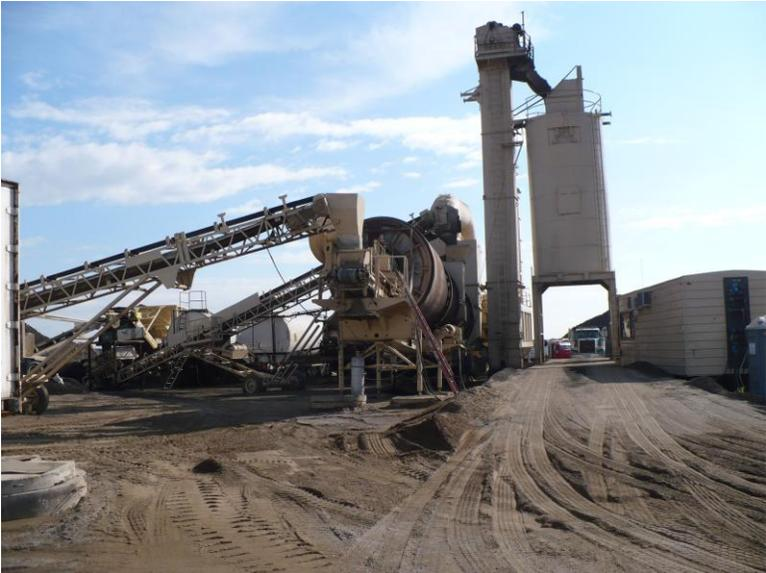
**Figure 16 FRAP productions: Conveyers, drum, elevator, and silo.**
