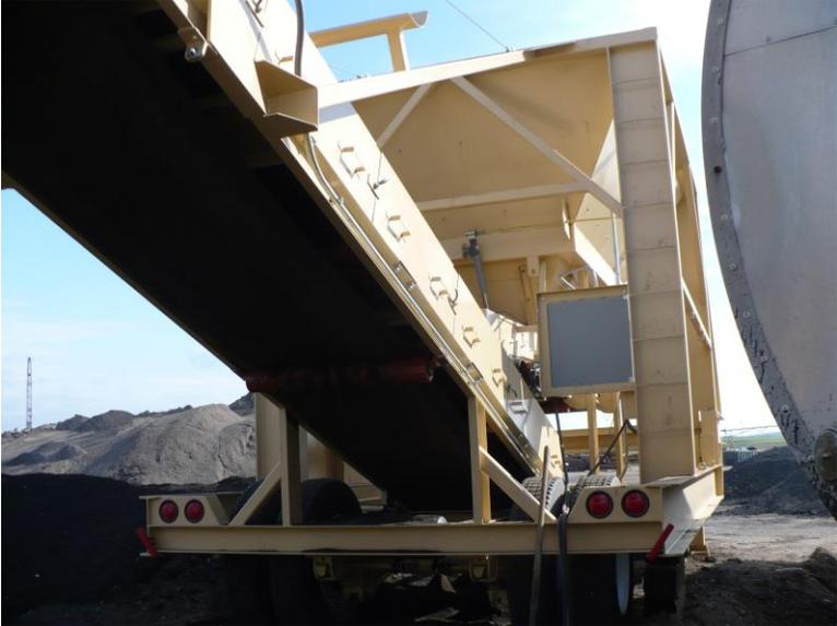
**Figure 15 FRAP production: Covered conveyor belt for fine RAP.**
