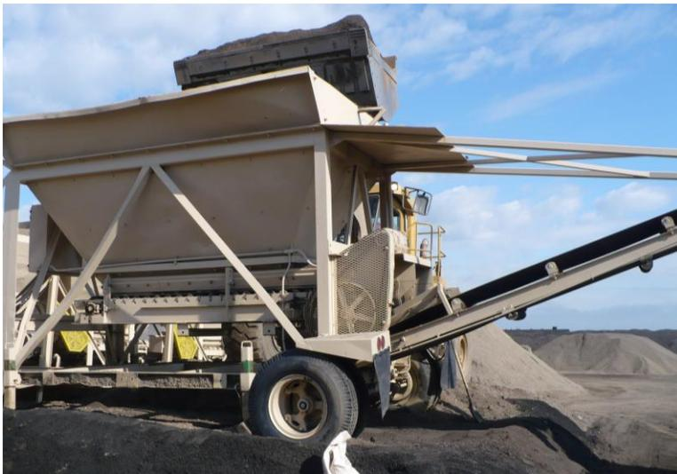
**Figure 14 FRAP production: Loader at RAP feed bin.**
