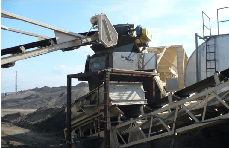
**Figure 17 FRAP production: Vibrating screen combining Fine and Coarse RAP.**
