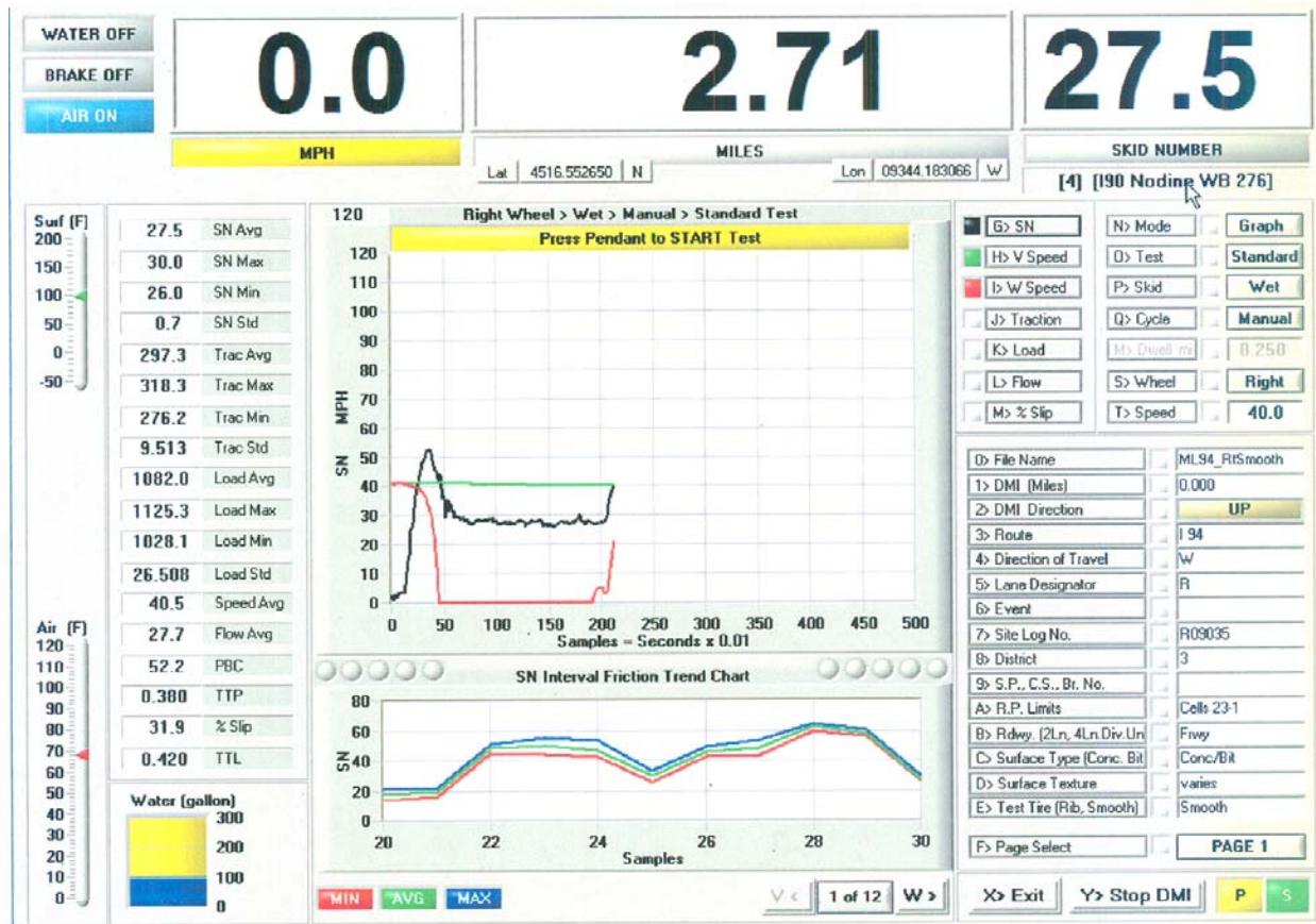
Figure 2. Screenshot of the Friction Testing Software in the Field
