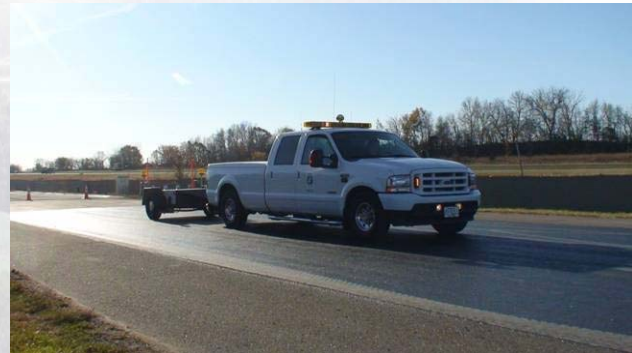
Figure 1. KJ Law (Dynatest) Skid Trailer
