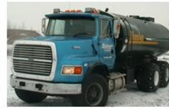
S1 (Homemade 4,400 gal-flotation tires)
