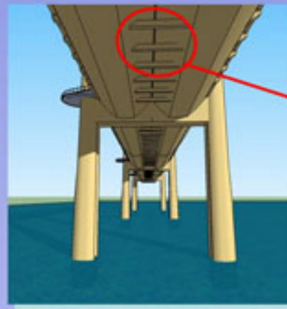
Two box girders
