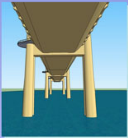
One box girder
