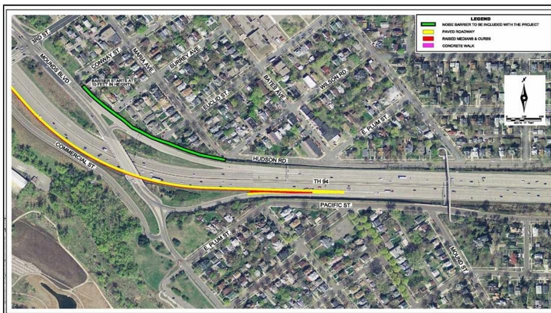
Figure 2. Mounds Boulevard noise barrier. New barrier E3 to be included with the project: Conway Street to Wilson Road/Hudson Road.
