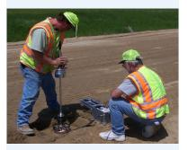
An LWD repeatedly drops a mass on a loading plate in contact with the ground to estimate its stiffness.
